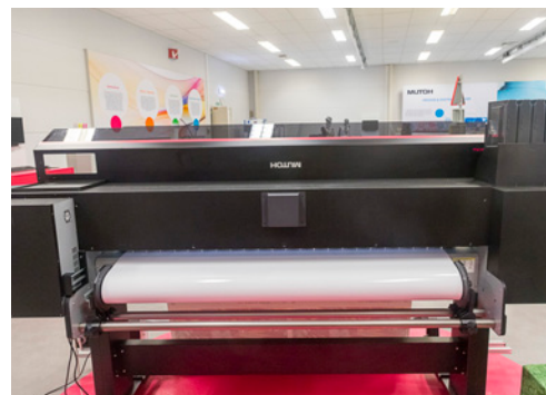
The distance between the feed roller and the print path is minimal.
