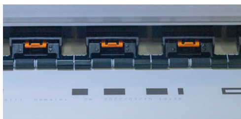
The printer keeps track of consumption and when changing rolls in the meantime, the printer prints this after which the code is read when the roll is placed again
